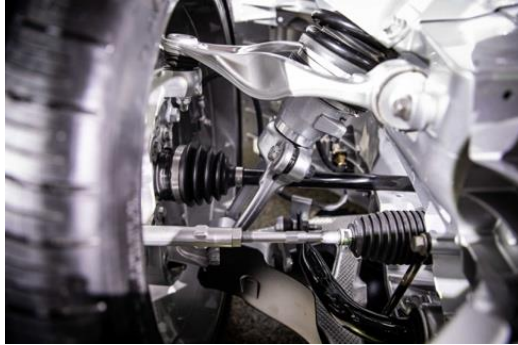
Slight adjustments to the Z06 front suspension geometry were necessary to make room for the front drive axle. Cameron Neveu
