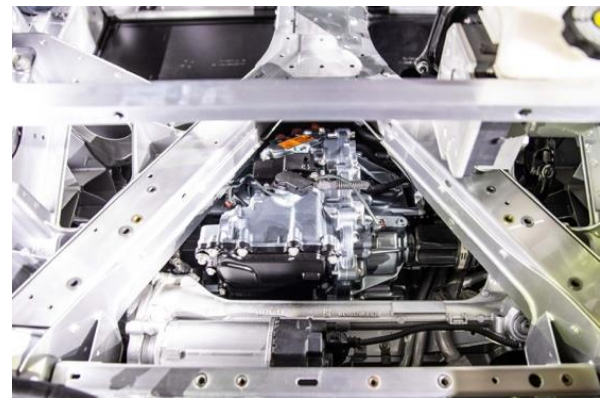
The E-Ray's front drive unit powers the battery—during braking, coasting, and normal driving—via an inverter. Cameron Neveu
